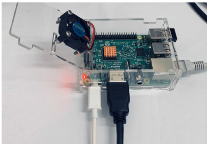
Fig. 7. Actual implementation on Raspberry Pi 3 Model B+ platform.
